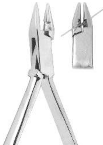
AURA-7-5135 Bird beak pliers for bending round, square or rectangular wire up to 0,7 mm. (.028"). With cutter.
